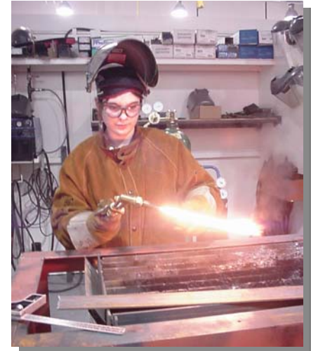
Grade 9 welding student, Rosalind Skinner starts the oxyacetylene cutting torch.
